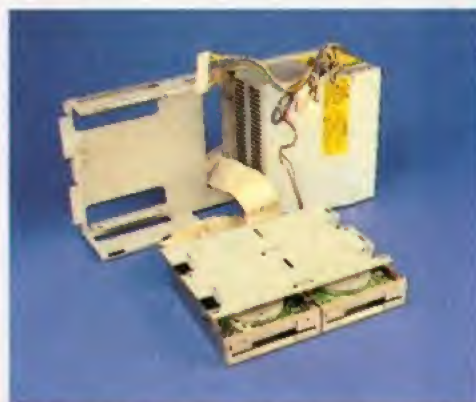
8 To fit the XL drive you will need to disassemble the drive and power subassembly. Detach the spacers from under the old drive and add them to the XL.
